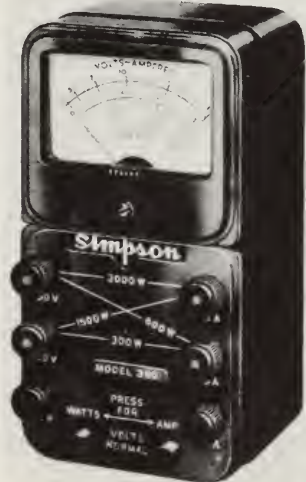
7-46. A combination volt, ampere, and watt meter. (Simpson Electric Co.)
